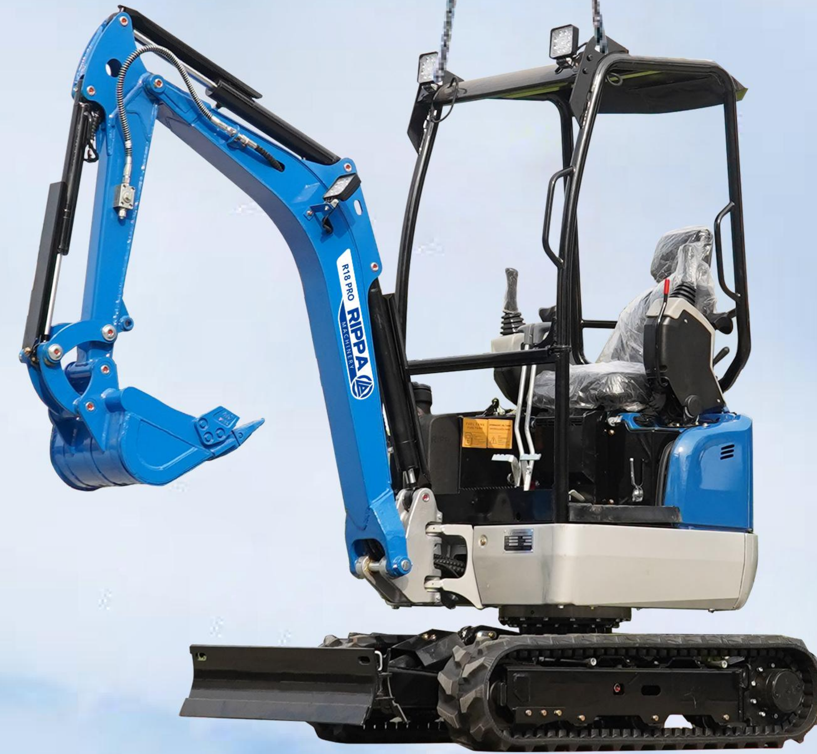
Arrive quickly at a new place of use: The lifting eyes integrated in the canopy enable simple and quick moving or loading of the machine by means of the practical two-point suspension.
